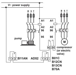
EXAMPLE OF ELECTRICAL WIRING
