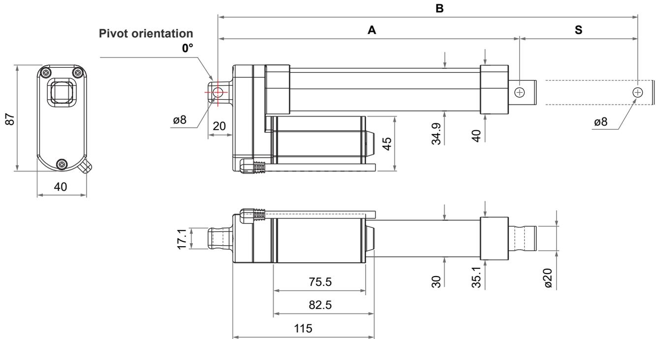
**Note:** As an example in 0° orientation for rear connector.
