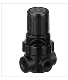
Parts Mounting orientation Working pressure min./max. Ambient temperature min./max. Medium temperature min./max. Medium Regulator type Regulator function Adjustment range min./max. Pressure supply Activation Weight Pressure regulator Any 0,5 ... 25 bar -10 ... 60 °C -10 ... 60 °C Compressed air Neutral gases Diaphragm-type pressure regulator with relieving air exhaust See table below single Mechanical See table below
