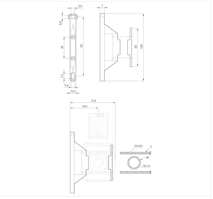
L = Mounting screw M = O-ring Efficient pneumatic solutions, our program: cylinders and drives, valves and valve systems, air supply management
