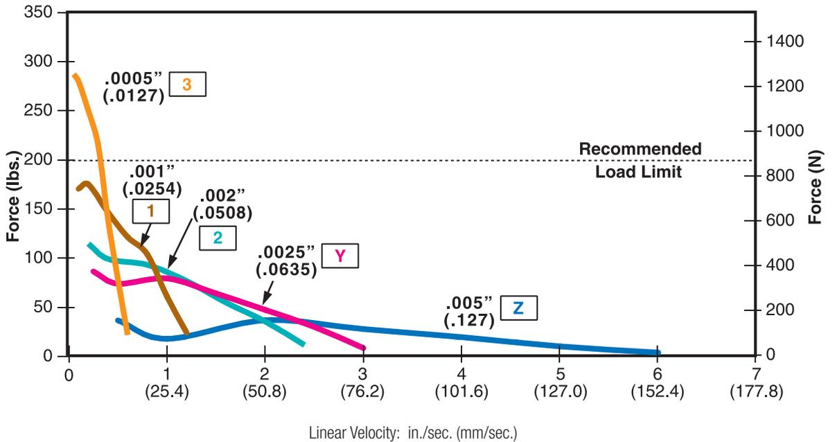
NOTE: All chopper drive curves were created with a 5 volt motor and a 75 volt power supply.
