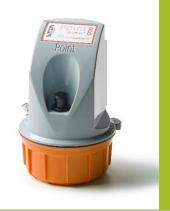
Point Orange 3G is a compact Logger/RTU device with integrated battery, a 3G modem with GPRS fallback, internal and/or external antenna, flexible I/O options, Modbus and SDI-12 master capability and a submersion sensor.
