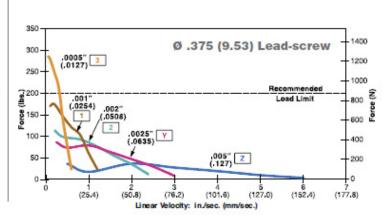
NOTE: All chopper drive curves were created with a 5 volt motor and a 40 volt power supply. Ramping can increase the performance of a motor either by increasing the top speed or getting a heavier load accelerated up to speed faster. Also, deceleration can be used to stop the motor without overshoot. With L/R drives peak force and speeds are reduced, using a unipolar drive will yield a further 30% force reduction.
