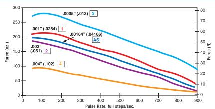
NOTE: All chopper drive curves were created with a 5 volt motor and a 40 volt power supply.
