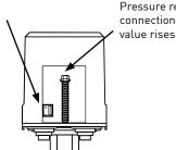
Pressure regulation at connection: pressure value rises on screwing
